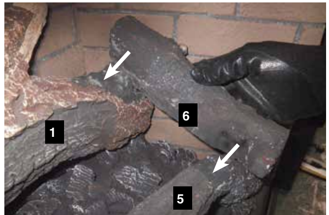
8. Line locator at top of Log 6 with provision on Log 1 - the locator at the bottom of Log 6 should line up with the provision on Log 5.
