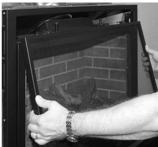
STEP 2: Locate the two small vertical studs on the firebox top. Slightly angle the screen upwards and line up the tab holes with the firebox studs.
